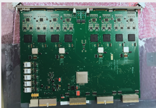
Fig. 1: FEB for the Calorimeter Upgrade in the LHCb experiment. Each one includes 8 ICECAL chips designed and produced by the ICCUB Technological Unit
